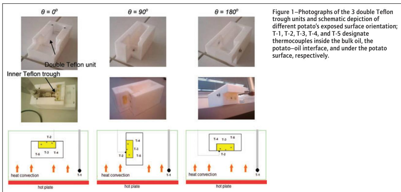
Figure 1—Photographs of the 3 double Teflon trough units and schematic depiction of different potato's exposed surface orientation; T-1, T-2, T-3, T-4, and T-5 designate thermocouples inside the bulk oil, the potato–oil interface, and under the potato surface, respectively.
