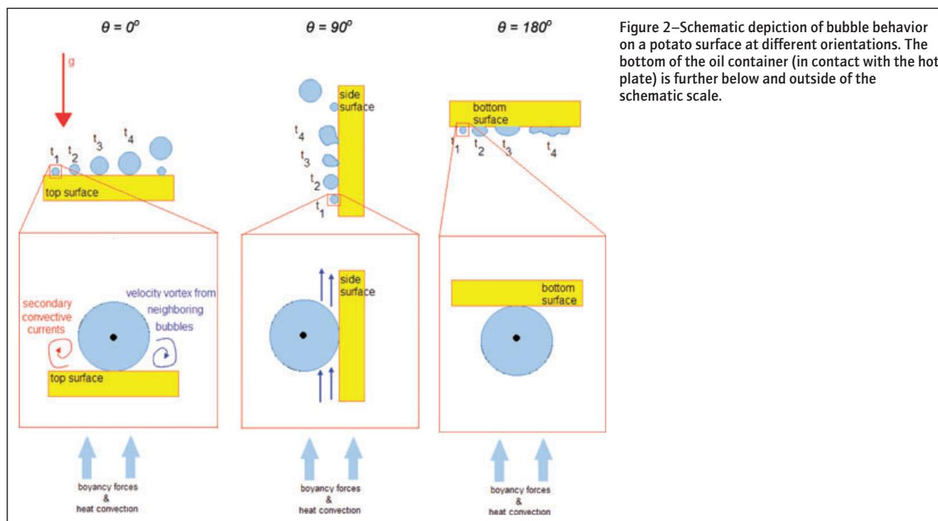
Figure 2—Schematic depiction of bubble behavior on a potato surface at different orientations. The bottom of the oil container (in contact with the hot plate) is further below and outside of the schematic scale.
