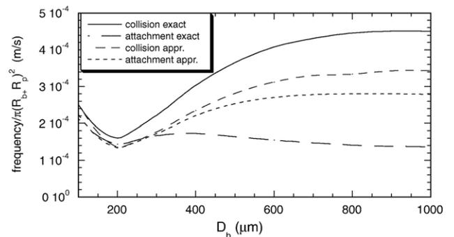
Fig. 7. Collision and attachment frequencies computed by Eq. (24) (exact) and by getting  $P$  out of the integral and computed it at the rms velocity values (approximate). (Parameters:  $D_p=10 \text{ }\mu\text{m}$ ,  $U_b=0$ ,  $u_p=0$ ,  $\varepsilon=1 \text{ m}^2/\text{s}^3$ ).
