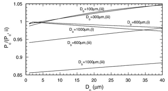
Fig. 1. Ratio between collision efficiency  $P_c$  from models (i) and (iii) to collision efficiency of model (ii) versus particle diameter  $D_p$  for several bubble sizes.
