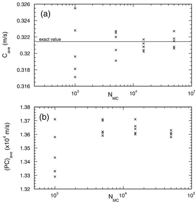
Fig. 5. Computed value of average total bubble–particle relative velocity  $C_{ave}$  for several Monte Carlo realizations with different number  $N_{MC}$  of computational points (a) ignoring efficiencies (b) including efficiencies (Parameters:  $D_p=10 \text{ }\mu\text{m}$ ,  $D_b=1000 \text{ }\mu\text{m}$ ,  $U_b=0$ ,  $u_p=0$ ,  $\varepsilon=1 \text{ m}^2/\text{s}^3$ ).
