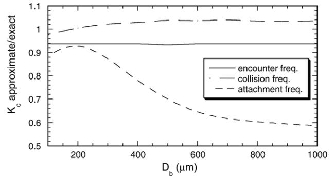
Fig. 6. Ratio between approximate (Eq. (24)) and exact (Eq. (21)) value of the encounter (i.e.  $P=1$ ), collision (i.e.  $P_a=1$ ) and attachment frequency  $K_c$  versus bubble diameter  $D_b$ . (Parameters:  $D_p=10 \text{ }\mu\text{m}$ ,  $U_b=0$ ,  $u_p=0$ ,  $\varepsilon=1 \text{ m}^2/\text{s}^3$ ).
