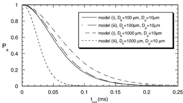
Fig. 2. Attachment efficiency  $P_a$  from models (i) and (iii) versus induction time  $t_{ind}$  for several pairs of bubble and particle diameters.
