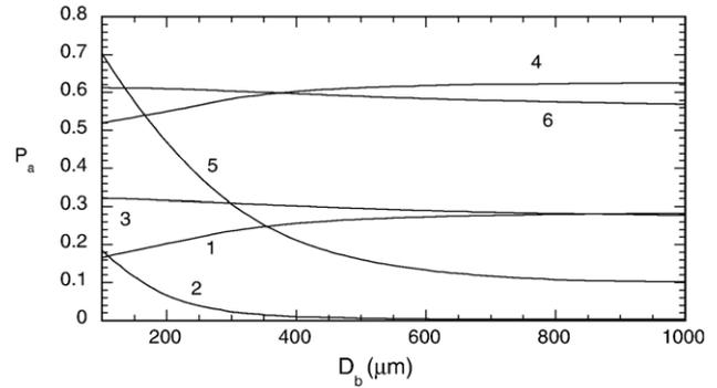
Fig. 3. Attachment efficiency versus bubble diameter  $D_b$ : (1) model (i),  $t_{ind} = 0.1 \text{ s}$ ,  $D_p = 10 \mu\text{m}$  (2) model (iii),  $t_{ind} = 0.1 \text{ s}$ ,  $D_p = 10 \mu\text{m}$  (3) model (ii),  $h_r = 1.98$ ,  $D_p = 10 \mu\text{m}$  (4) model (i),  $t_{ind} = 0.02 \text{ s}$ ,  $D_p = 30 \mu\text{m}$  (5) model (iii),  $t_{ind} = 0.02 \text{ s}$ ,  $D_p = 30 \mu\text{m}$  (6) model (ii),  $h_r = 1.45$ ,  $D_p = 30 \mu\text{m}$ .
