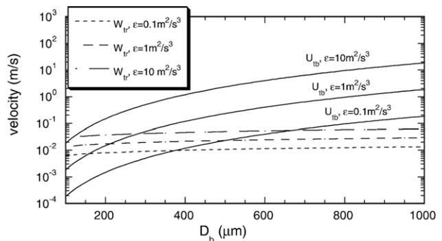
Fig. 4. Rms of relative bubble–fluid ( $U_{tb}$ ) and bubble–particle ( $W_{tr}$ ) turbulence induced velocities versus bubble diameter  $D_b$  for three values of turbulent energy dissipation rate  $\varepsilon$  ( $D_p = 10 \mu\text{m}$ ).
