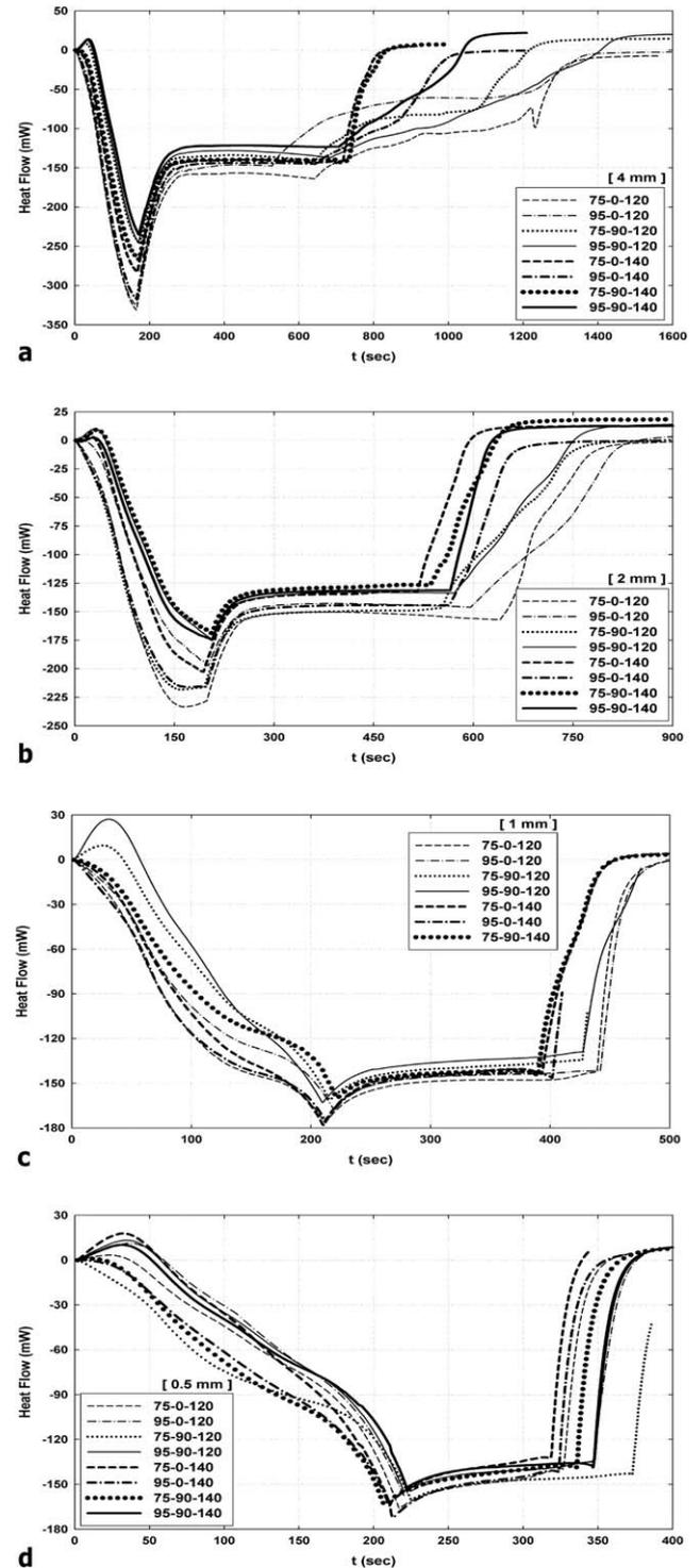
Fig. 4. Heat flow versus time for all the examined conditions and for films of varying thickness: (a) 4 mm, (b) 2 mm, (c) 1 mm and (d) 0.5 mm.
