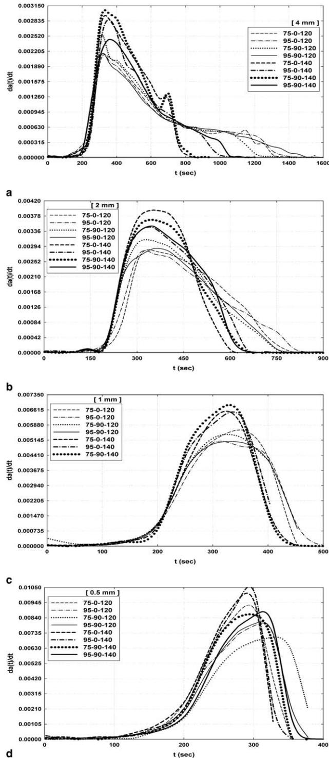
Fig. 3. Normalized drying rate,  $d\alpha(t)/dt$ , versus time for all the examined conditions and for films of varying thickness: (a) 4 mm, (b) 2 mm, (c) 1 mm and (d) 0.5 mm.
