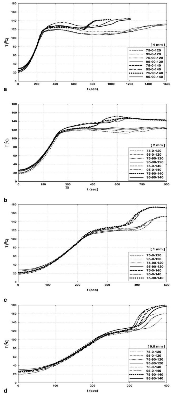
Fig. 1. Temperature profiles for all the examined conditions and for films of varying thickness: (a) 4 mm, (b) 2 mm, (c) 1 mm and (d) 0.5 mm.
