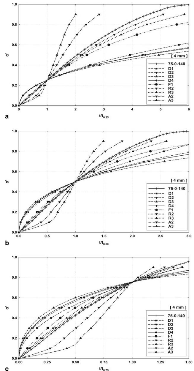
Fig. 5. Reduced-time plot of degree of loss-in-weight,  $\alpha'$ , versus (a)  $t/t_{0.25}$ , (b)  $t/t_{0.50}$  and (c)  $t/t_{0.75}$  along with theoretical curves calculated for various solid-state reaction equations. The plotted data are quasi-isothermal measurements from the run with a 4 mm film thickness,  $75\text{ }^\circ\text{C}$  pasting temperature, 0 min pasting duration and  $140\text{ }^\circ\text{C}$  drying temperature. Symbols explained in Table 1.
