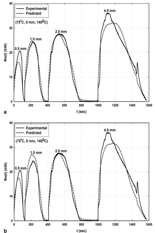
Fig. 6. Regression results based on Eq. (5) against experimental data for films with thickness 0.5, 1, 2 and 4 mm film and for 75 °C pasting temperature, 0 min pasting duration and 140 °C drying temperature: (a) with the specific load term and (b) without the specific load term (case #37 in Table 3).
