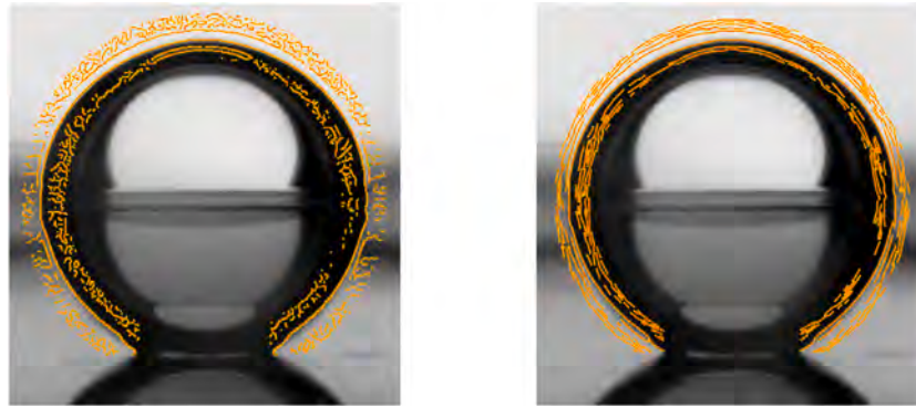
Fig. 9. Comparison of the detected edges (orange lines) for the conventional Canny method (left) with the proposed advanced method for bubble shapes (right). The edge detection is just performed close to the bubble's interface (see Fig. 10(c)).
