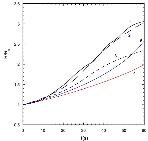
**Fig. 10.** Bubble radius evolution curves: (1) Experimental (2) Variable vapor pressure (3) Variable vapour pressure with no mass transfer contribution (4) Vapor pressure 1 bar (5) Vapour pressure 1.1 bar.
