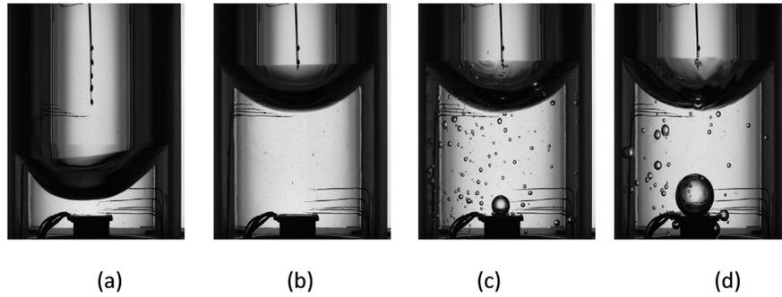
**Fig. 2.** Pictures of the different sequences of the experiment: (a) tank filling;  $t = 73$  s, (b) Marangoni convection at the free surface;  $t = 155$  s, (c) subcooled boiling;  $t = 240$  s, (d) saturated boiling;  $t = 370$  s.
