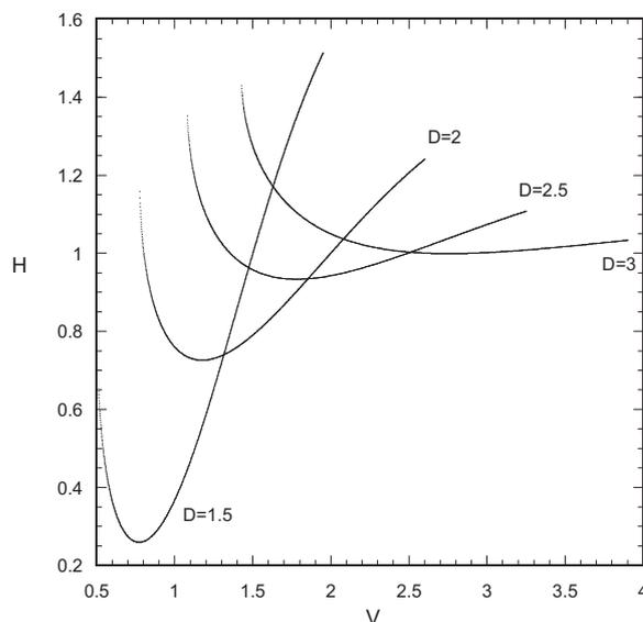
Fig. 2. Dependence of liquid bridge pressure  $H$  on total bridge volume  $V$  for several values of length  $D$ .
