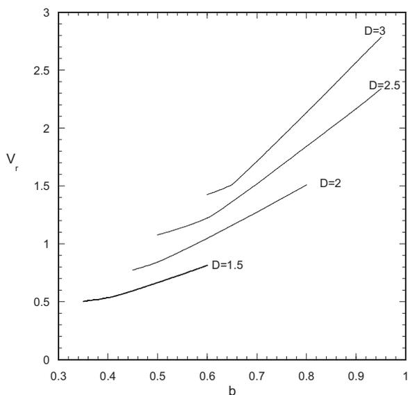
**Fig. 3.** Total bridge volume  $V_r$  at the rupture point vs bubble radius  $b$  for several values of length  $D$ .
