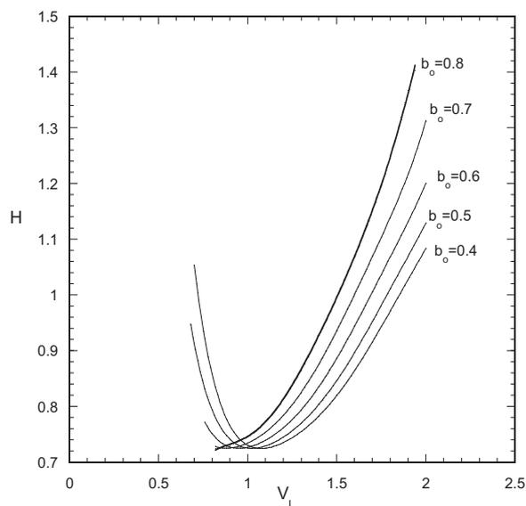
**Fig. 6.** Evolution of pressure  $H$  in the bridge vs liquid volume  $V_L$  for  $D=2$  and several values of initial bubble radius  $b_0$  in the limit  $B \gg 1$ .
