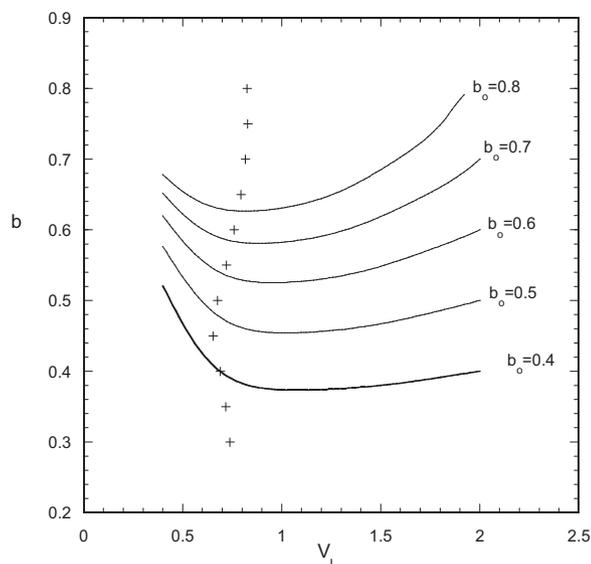
**Fig. 5.** Evolution of the bubble radius  $b$  vs liquid volume  $V_L$  for  $D=2$  and several values of initial bubble radius  $b_0$  in the limit  $B \gg 1$ . The crosses designated the rupture location.
