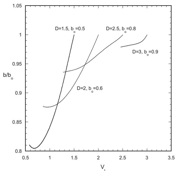
**Fig. 4.** Evolution of the bubble radius  $b$  vs liquid volume  $V_L$  for several pairs of length  $D$  and initial bubble radius  $b_0$  in the limit  $B \gg 1$ .
