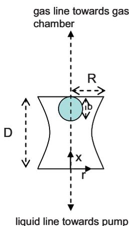
Fig. 1. Schematic of the liquid bridge-bubble system.
