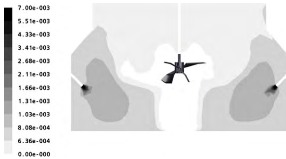
Fig. 6. Case I: Vertical map of the contours of mud particles concentration [kg/kg water], in the absence of coagulation. 7 \times 10^{-3} kg/kg water is the mud concentration at the entrance of the recycling streams.
