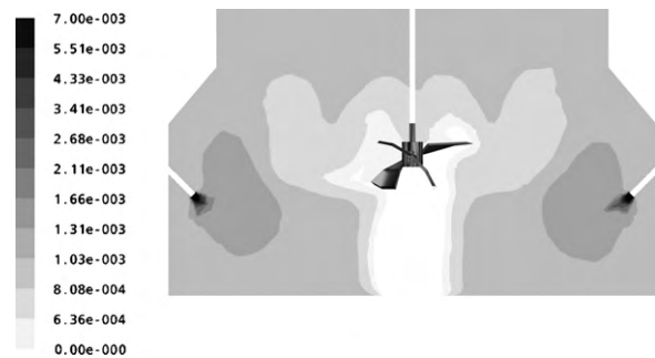
Fig. 10. Case III: Vertical map of the contours of mud particles concentration [kg/kg water].
