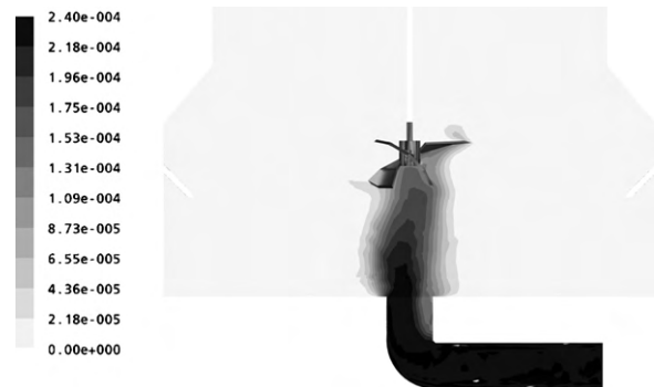
Fig. 9. Case III: Vertical map of the contours of fresh particles concentration [kg/kg water].
