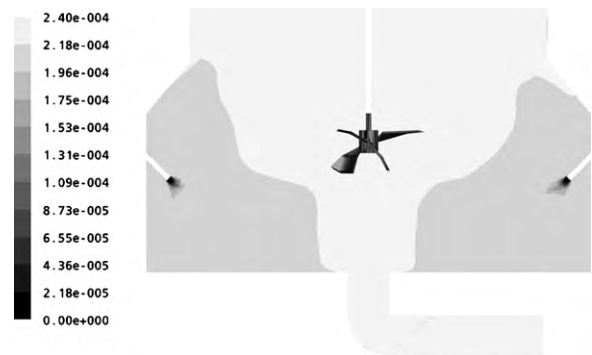
Fig. 5. Case I: Vertical map of the contours of fresh particles concentration [kg/kg water], in the absence of mud particles and polyelectrolyte. The floc concentration entering with the water mainstream at the bottom of the tank is 2.4 \times 10^{-4} kg/kg water.
