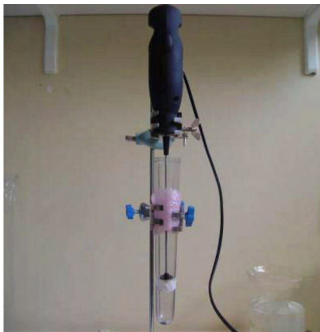
Fig. 1. Emulsification set-up. Coffee creamer is on top with Plexiglas taper vessel underneath.
