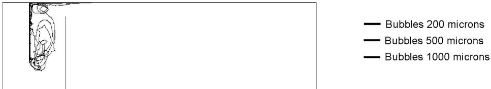
**Figure 12** Bubble trajectories: bottom vertical injection
