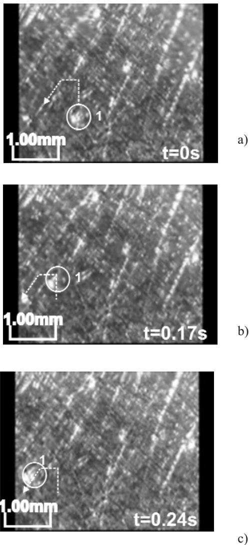
Figure 5: Bubble motion over the scratched disk heater (a)  $t=0\text{s}$ , (b)  $t=0.17\text{s}$  and (c)  $t=0.24\text{s}$   $T_{\text{thermistor}}=40^\circ\text{C}$ , (1 g).
