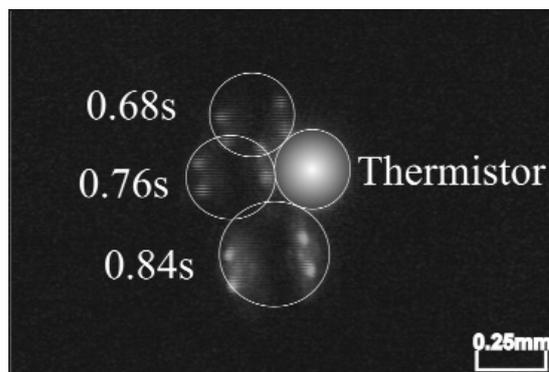
Figure 2: Instants during bubble displacement across the surface of the spherical heater (thermistor),  $T_{\text{thermistor}} = 45^{\circ}\text{C}$ , ( $\sim 0$  g).
