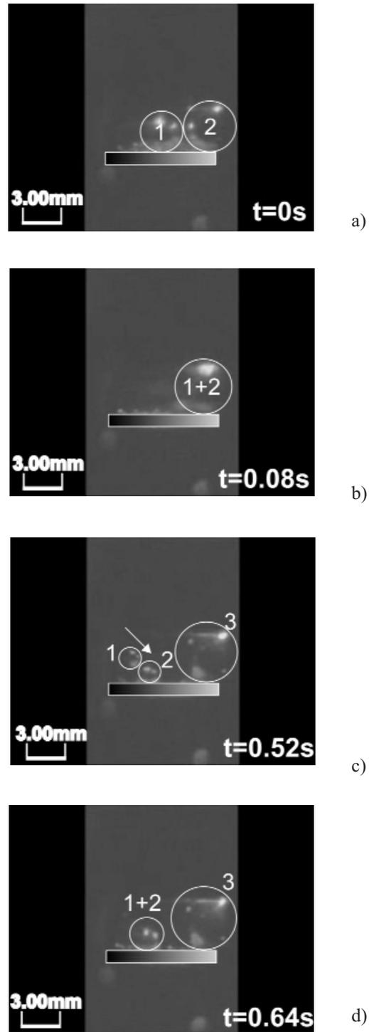
Figure 7: Coalescence of bubbles over the smooth plate heater, (a)  $t=0\text{s}$ , (b)  $t=0.08\text{s}$ , (c)  $t=0.54\text{s}$  and (d)  $t=0.64\text{s}$ ,  $T_{\text{thermistor}}=50^{\circ}\text{C}$ , ( $\sim 0$  g).
