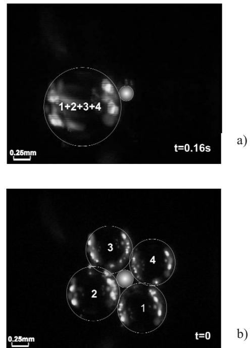
Figure 6: Coalescence of four (4) bubbles attached to the spherical heater at (a)  $t=0\text{s}$  and (b)  $t=0.16\text{s}$ ,  $T_{\text{thermistor}}=80^\circ\text{C}$ , ( $\sim 0\text{ g}$ ).
