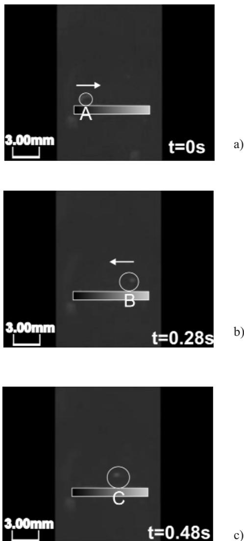
Figure 3: Bubble motion over the smooth plate heater (a)  $t=0s$ , (b)  $t=0.28s$  and (c)  $t=0.48s$ ,  $T_{thermistor}=40^{\circ}C$ , ( $\sim 0g$ ).
