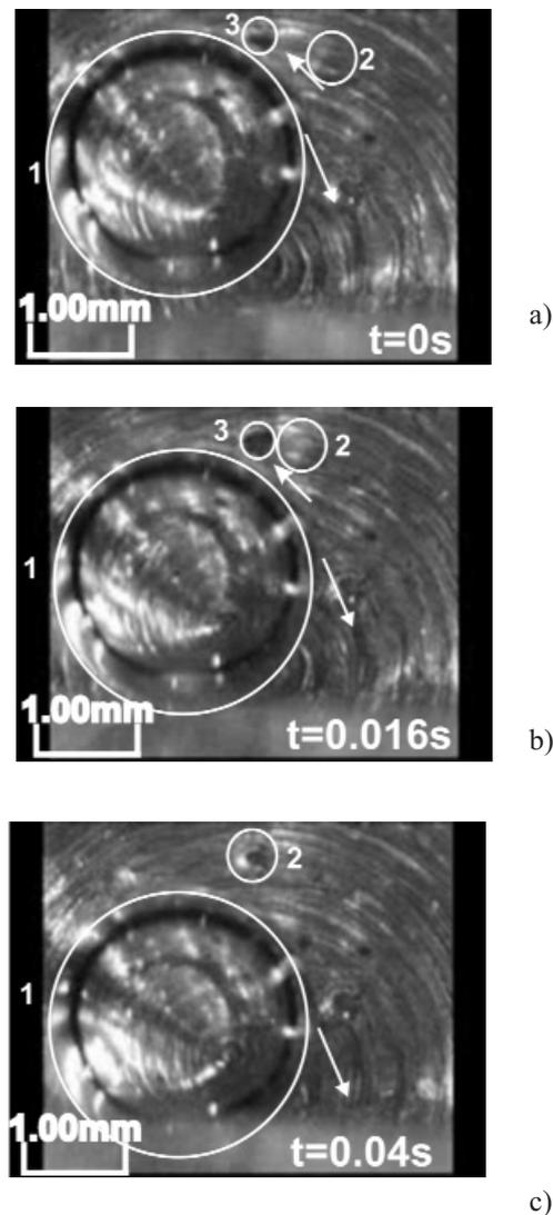
Figure 4: Bubble motion over the circular grooved disk heater; (a)  $t=0s$ , (b)  $t=0.016s$  and (c)  $t=0.04s$ ,  $T_{thermistor}=40^{\circ}C$ , ( $1g$ ).
